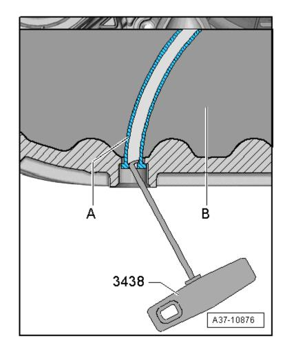
Press new fluid level pipe -A- into ATF inspection hole -B- by hand.
