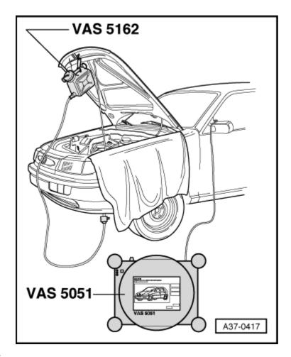
Remove O-ring -1- at connection -2- on ATF charging device for CVT gearboxes -VAS 5162-.
