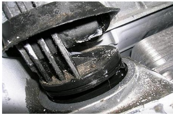
Figure 2. Dust cover lifted to view the sealing area.
