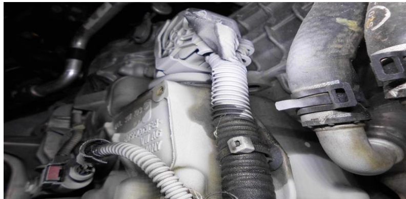
Figure 1. Evidence of oil leak from the transmission control module seal.
