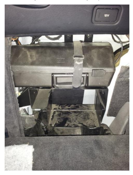
Passenger side amp. At first I thought I had to remove the whole amp, but fortunately removing the head unit was enough to get comfortably to the screws.
