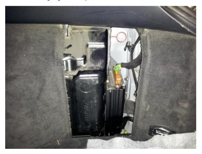
CD changer bracket completely removed, great access to the screws.
