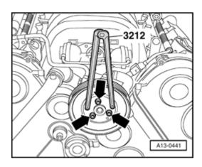
Remove ribbed belt gear of power steering pump (arrows) using spanner wrench 3212 as retainer.
