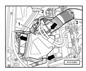
Disconnect Evaporative Emission (EVAP) canister purge regulator valve N80 - 1 - at air filter housing.
