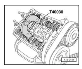
= Insert camshaft adjuster gauge T40030 at camshafts of right cylinder head.
