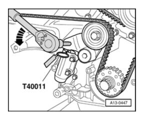
Using an 8 mm socket head wrench, turn toothed belt tensioning roller in direction of arrow until pin T40011 can pulled out.
