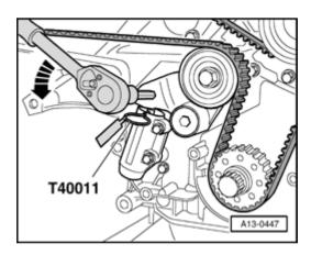
Using an 8 mm hex socket wrench, turn toothed belt tensioner in direction of arrow until tensioning lever pushes tensioner together far enough so that pin T40011 can be inserted into hole of pistons and housing.
