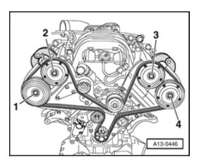
Loosen but do not remove bolts - 1 - to - 4 - for camshaft gears.
