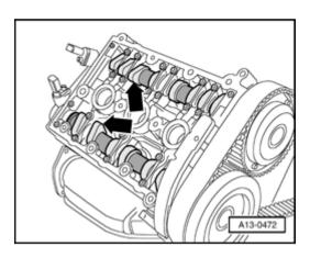
Turn engine until cams (arrows) at intake and exhaust camshaft of cylinder 3 (right cylinder bank) point upward uniformly.
