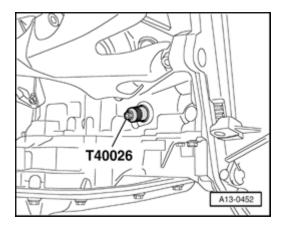
Thread locking pin T40026 into hole of removed sealing plug and tighten.
