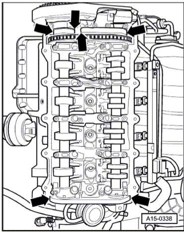
Tighten cylinder head cover in sequence -12 to 1-.
