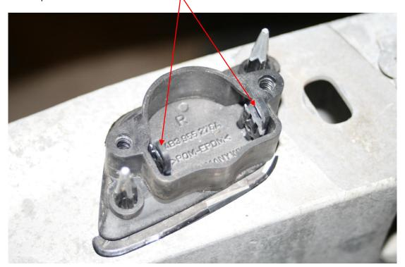
Here's the assembly, off of the bumper, with the center bracket turned 180 degrees to release the tension in the spring and the coverplate removed:
