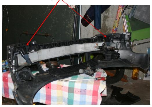
The washers are held on the bumper with two screws and a bracket. The assembly is spring loaded, so it won't come apart with the two screws removed.
