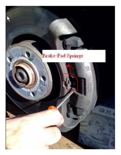
Just use a screwdriver and pull up. It is a big 'S' with clips on both ends. Be careful is will just jump out. Some folks have broken this spring when yanking it out – go to the local stealership for replacement if you break it.
