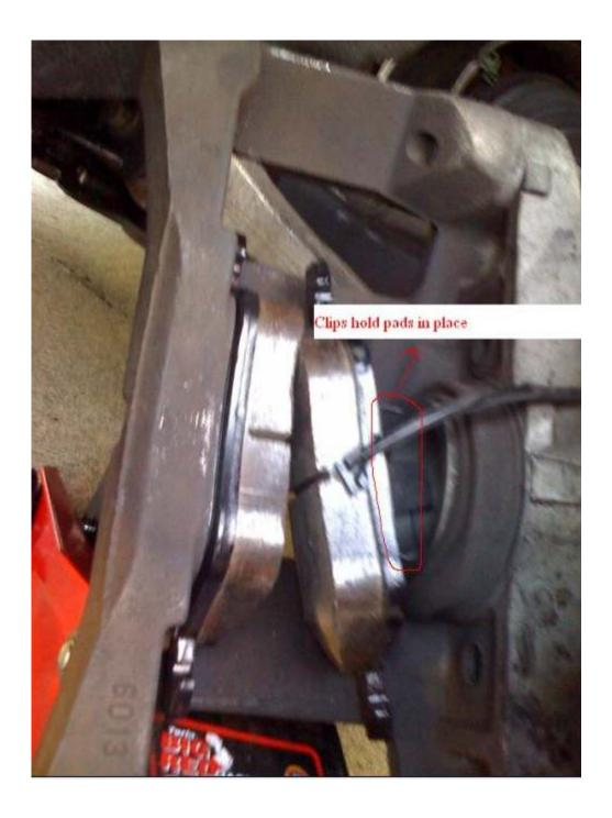
If changing only the pads, put the caliper back onto the rotor and use the 7mm hex key to tighten the two screws (torque: 30Nm; about 18 lb-ft) - and then put the 'S' spring in place. Fill in the brake fluid reservior to correct level.
