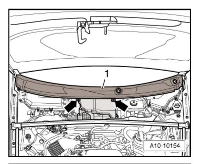
Remove bolts -arrows- and remove cover for E-box at right in engine compartment.
