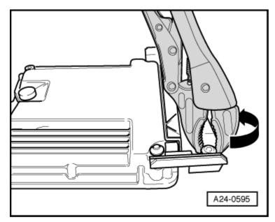
The threads of both shear bolts -3- that are installed in the ECM are not coated with a locking compound. The threads in the ECM housing must not be heated and do not require to be heated (unintentional heating of the ECM).
