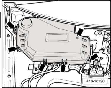
Carefully pry off retaining clip -2- with a screwdriver -arrows 1 and 2- and remove ECM from E-box.
