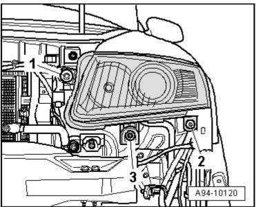
Adjust headlight -2- so that the distance -ato the spacer -1- is the same distance as measured upon removal.
