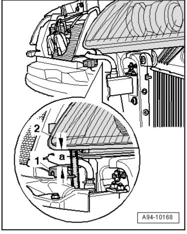
Make sure to counterhold adjuster nuts -1- of adjusters when unscrewing securing bolts to prevent them from being turned out of position - arrows-
