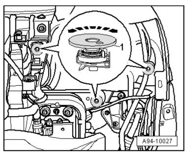
Fit headlight and screw in bolts -1 ... 3- two complete turns each.
