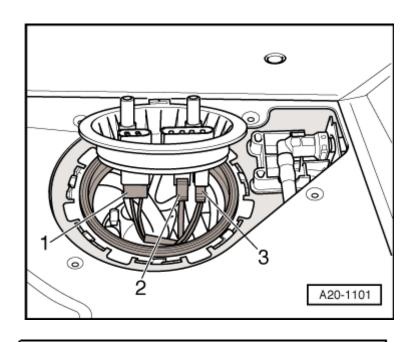
To separate the line couplings that are mentioned later in the description, pull the fuel lines out of the fuel tank opening.
