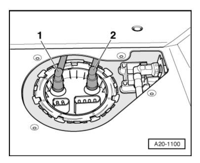
Connect electrical harness connectors -1and -2- to right locking flange.
