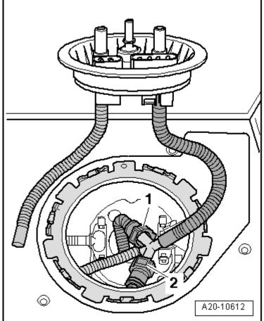
Through the left opening in the fuel tank, press the release button and disconnect the overflow line -1-, the suction jet line -2
