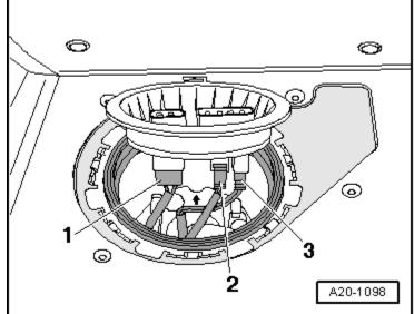
• The tab -2- on locking flange must lie between tabs -1- and -3- on fuel tank.
