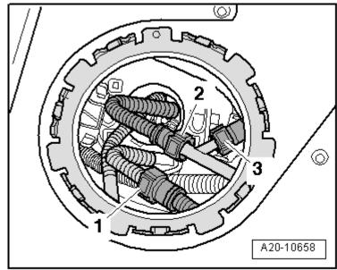
Install the fuel supply line -2- through the right opening in the fuel tank until it audibly engages.
