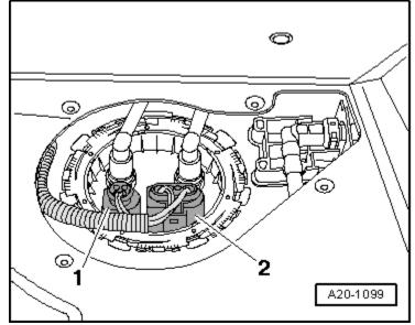
Mark the fuel return line -1- and fuel supply line -2-.
