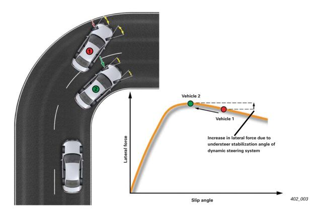
Most drivers react to this situation by applying more steering lock (vehicle 1). This reduces the available lateral friction between the tires and road surface. The static friction between the tires and road surface becomes sliding friction which causes the vehicle to lose control and leave the road. In this situation, corrective intervention by the ESP system will often be of no use.
