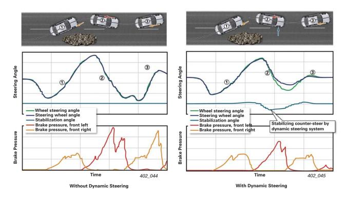
With the dynamic steering system, stabilizing countersteer is applied automatically, without the driver noticing anything. This significantly reduces the steering effort required on the part of the driver. The driver need only apply the steering angle that would be necessary in a similar, stable driving situation.
