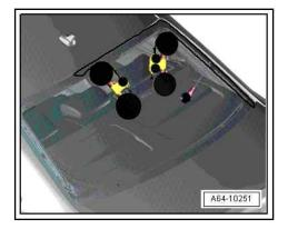
Cut window clear upwards along D-pillar.
