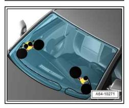
Insert end of cutting wire -1- into reel -2-.
