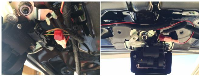
One to each of the two middle wires connecting to the push button. (Brown, and Blue\Yellow wires)
