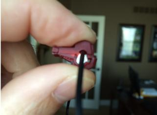
6. Install the three red wire taps onto the existing wiring. The locations are as follows:
