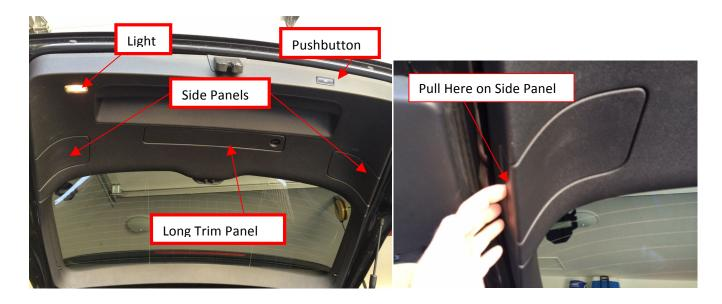
3. With someone to assist you pull the rear panel off the tailgate from the outside edge inward. There are several metal spring clips that just pull out as you gently pull the panel away from the tailgate.
