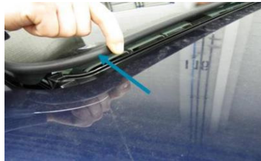
Figure 8. Seal for sunroof panel.
