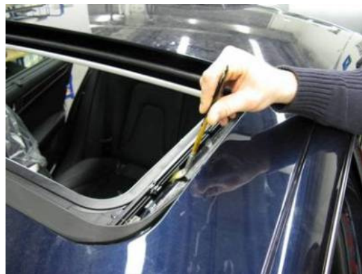
Figure 11. Outer guide rail.
