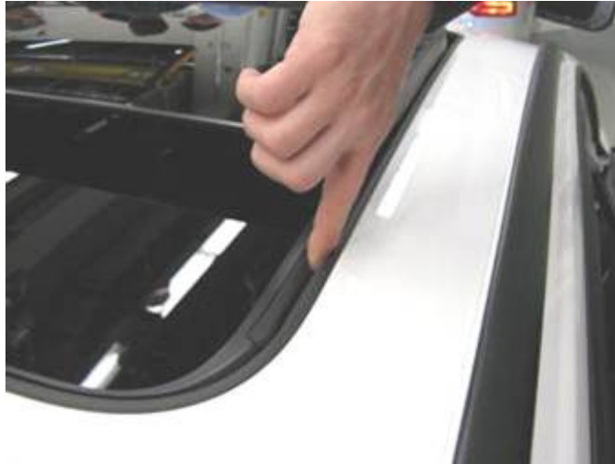
Figure 3. Seal for sunroof panel 2.
