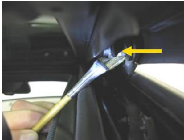
Figure 7. Locking pin for sunroof panel 1, viewed with panel 1 in a tilted position.
