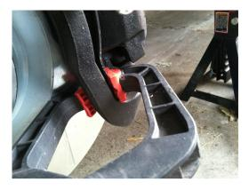
Now that you have the bottom clamped in place, I used an old 3/8 extension, because it provided enough height to pass of the lip of the brake pad
