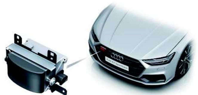
Laser Distance Regulation Control Module J1122
