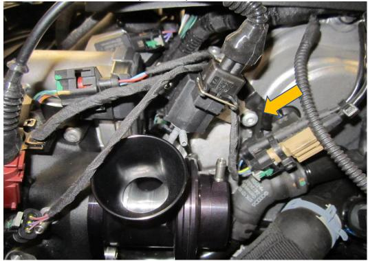
9. The Vacuum source is taken from the vacuum line that connects to the vacuum pump, cut the vacuum line as pictured below and fit the brass T-Piece provided.
